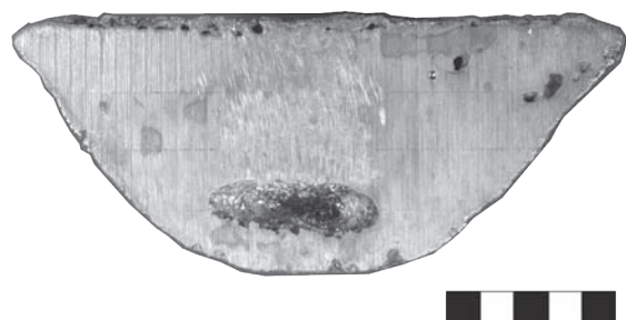
FIGURE 6. A cross-section of the ingot showing a large air bubble at the bottom.
